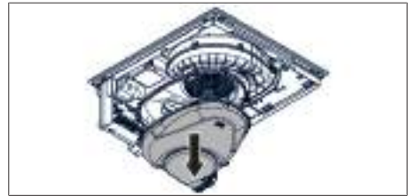
Fig. 11.28 Removing the bottom of the suction chamber
